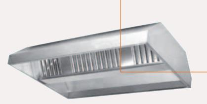
Monobloc construction in 18/10 AISI 304 stainless steel with Scotch-Brite® finishing, complete with motorfan 420 W 230 V (for mod. Ho3P1V-2V). The rectangular cross section provides better fume control and extraction.
